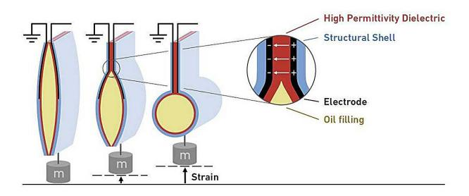
The diagram shows how the artificial muscle works and how the new shell is structured. Credit: Gravert et al. Science 2024 / ETH Zurich
