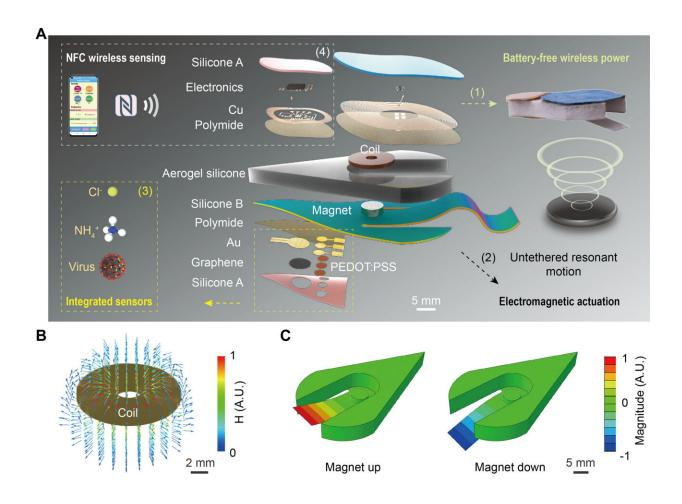
Architecture and functions of a battery-free wireless SES monitoring system. (A)
