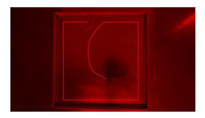
Researchers have developed a new soft robot design that engages in three simultaneous behaviors: rolling forward, spinning like a record, and following a path that orbits around a central point. The device, which operates without human or computer control, holds promise for developing soft robotic devices that can be used to navigate and map unknown environments. This image shows the path the robot took to map the boundary of a confined space. Credit: Jie Yin, North Carolina State University
