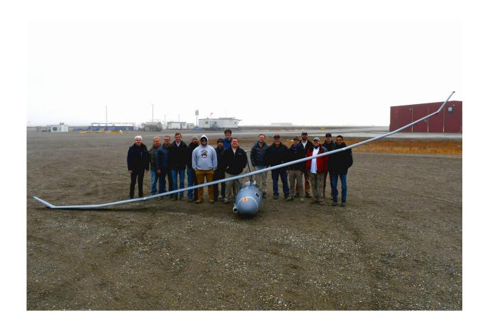
A team of researchers from Platform Aerospace, the Naval Postgraduate School (NPS) and the Naval Research Laboratory (NRL) recently used a Platform "Vanilla" unmanned aerial vehicle (UAV) to conduct testing of flight-path planning software developed at NPS. The flight tests above the Arctic Circle employed NPS' "POTION" software, which is intended to optimize the operational efficiency and endurance of manned and unmanned aircraft. Credit: U.S. Navy
