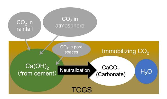
Infographic showing how aeration curing helps neutralize the alkaline nature of soil through carbon dioxide immobilization. Credit: Shinya Inazumi, SIT, Japan
