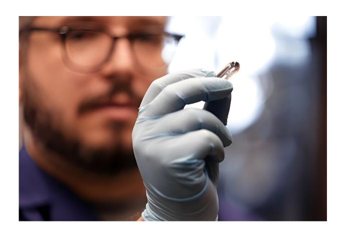
Abdon Pena-Francesch holds the soft gel before it is treated with chemicals that give the material its magnetic properties. The colorless precursor can be molded into a variety of shapes—such as capsules that could one day be ingested to deliver medicine. Credit: Brenda Ahearn/Michigan Engineering
