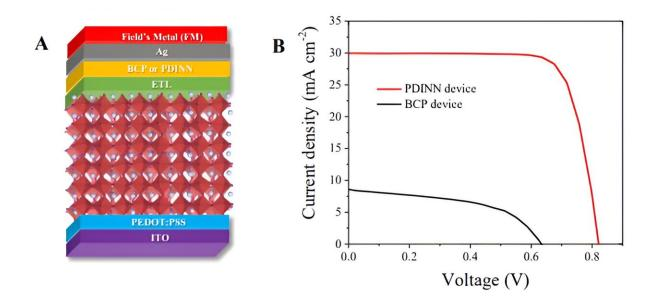
(A) Structure of a PV device with additional FM deposition. (B) J–V characteristics of PV devices with an FM layer under AM 1.5G one-sun illumination. Credit: *Advanced Energy Materials* (2023). DOI: 10.1002/aenm.202302555
