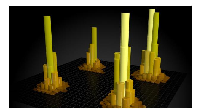
Scientific visualization of Bragg diffraction peaks in a 15x15 pixel patch of an undeformed bi-crystal gold sample. The height denotes photon counts. This data was acquired at the APS and processed on ALCF supercomputers. Credit: Argonne National Laboratory
