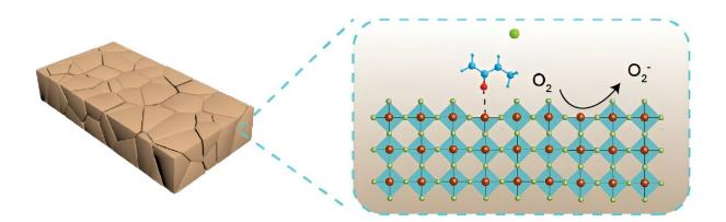
Schematic illustration of the effects of SEM-HCl additive on the tin perovskites. Credit: Wenbo Jia, Yi Jing, Han Zhang, Baoyan Tian, Huabo Huang, Changlei Wang, Ligang Xu
