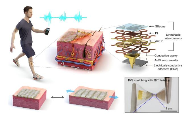
Design and working concept of the Stretchable microNeedle Adhesive Patch (SNAP). (A) Schematic illustration showing the overall system configuration and application of SNAP. (B) Exploded view schematic diagram of a SNAP, consisting of stretchable serpentine interconnects, Au-coated Si microneedle, and ECA made of Ag flakes–silicone composite. (C) Optical images showing high mechanical compliance of SNAP. Credit: The Korea Advanced Institute of Science and Technology (KAIST)
