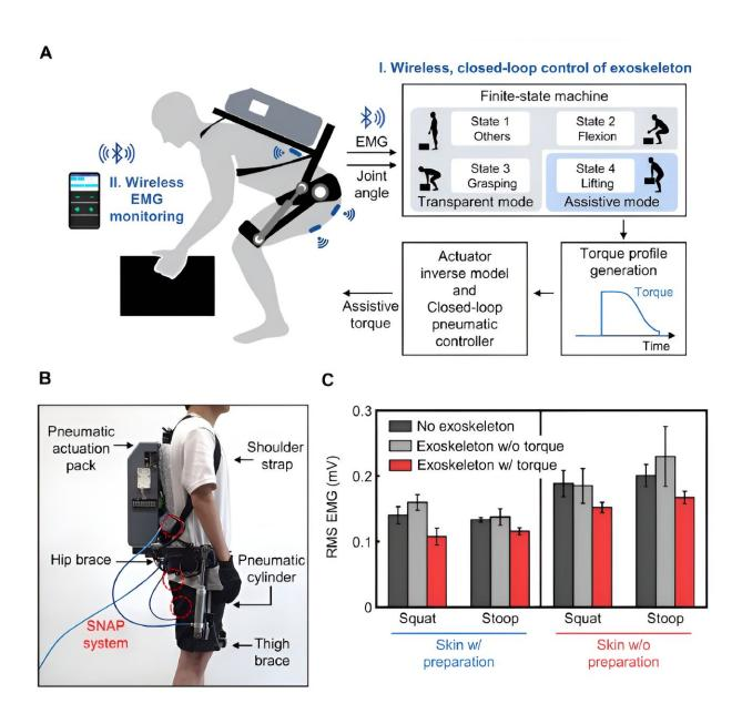
Demonstration of the wireless Stretchable microNeedle Adhesive Patch (SNAP) system as an Human-machine interfaces (HMI) for closed-loop control of an
