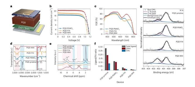
Photovoltaic performance and surface characteristics of PQD layers by different ligand exchange methods. Credit: *Nature Energy* (2024). DOI: 10.1038/s41560-024-01450-9
