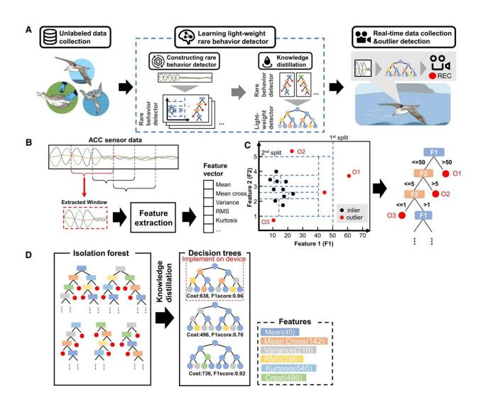
Overview and procedures of our method. A) Method overview. B) Feature extraction from sensor data and construction of a feature vector using a sliding time window. C) Outlier detection with an isolation tree. D) Decision trees are constructed from the isolation forest by knowledge distillation. From the trees,
