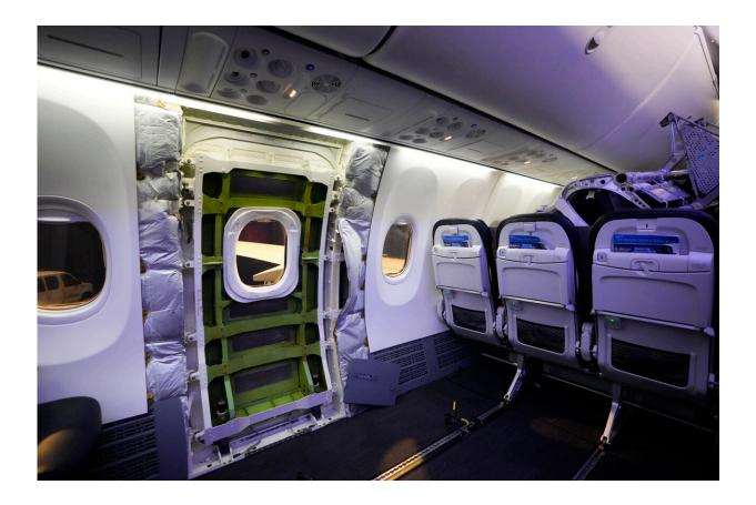
A door plug area of an Alaska Airlines Boeing 737 Max 9 aircraft awaiting inspection is pictured with paneling removed at the airline's facilities at Seattle-Tacoma International Airport on Jan. 10, 2024, in SeaTac, Wash. Boeing 737 Max 9 jetliners will carry passengers in the United States again, starting this weekend, for the first time since they were grounded after a panel blew out of the side of one of the planes. Credit: AP Photo/Lindsey Wasson, File
