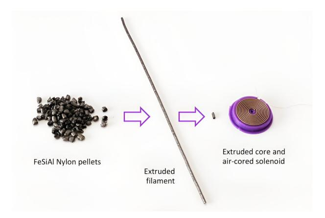
Solenoids are produced by precisely layering three different materials — a dielectric material that serves as an insulator, a conductive material that forms the electric coil, and a soft magnetic material that makes up the core. The soft
