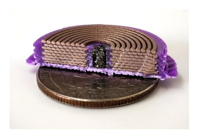
MIT researchers modified a multi-material 3D printer so it could produce threedimensional solenoids in one step by layering ultrathin coils of three different materials. It prints a U.S. quarter-sized solenoid as a spiral by layering material around the soft magnetic core, with thicker conductive layers separated by thin insulating layers. Credit: Massachusetts Institute of Technology
