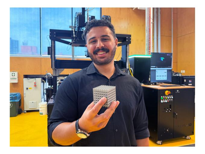
Ph.D. candidate Jordan Noronha holding a sample of the new titanium lattice structure 3D printed in cube form. Credit: RMIT.
