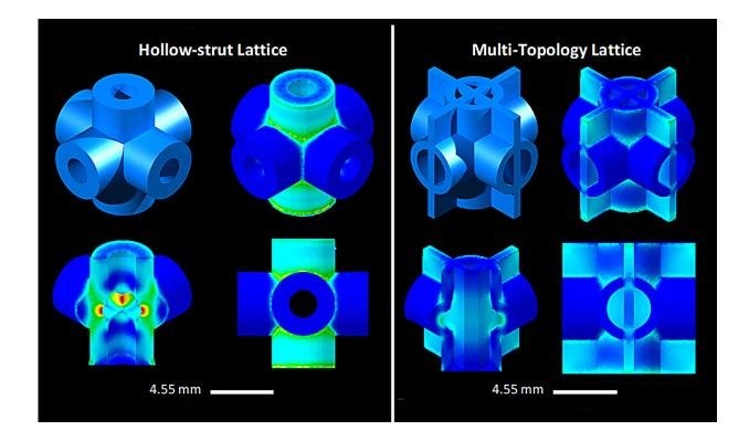
Compression testing shows (left) stress concentrations in red and yellow on the hollow strut lattice, while (right) the double lattice structure spreads stress more evenly to avoid hot spots. Credit: RMIT
