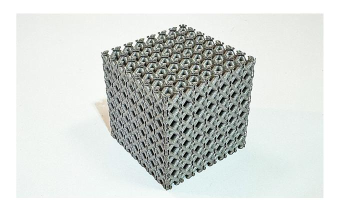
A sample of the new titanium lattice structure 3D printed in cube form. Credit: RMIT
