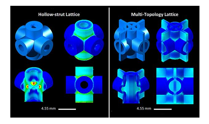
Compression testing shows (left) stress concentrations in red and yellow on the hollow strut lattice, while (right) the double lattice structure spreads stress more evenly to avoid hot spots. Credit: RMIT
