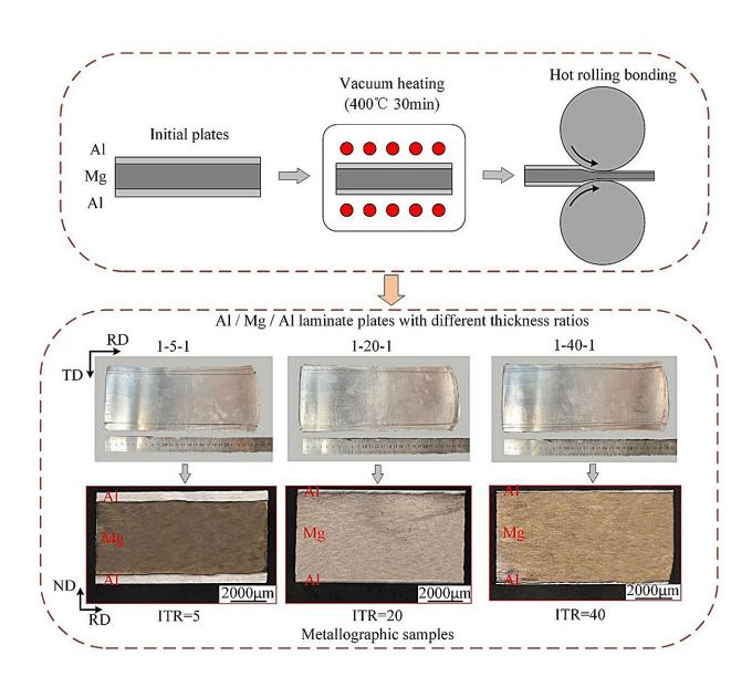
Schematic diagram of large thickness ratio Al/Mg/Al laminate rolling process.
