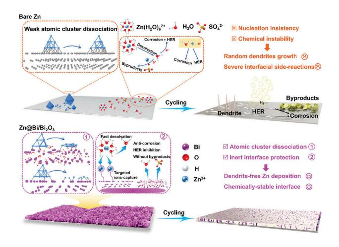
Illustration of ions-deposition behavior and interfacial chemistry on bare Zn (upper) and Zn@Bi/Bi<sub>2</sub>O<sub>3</sub> electrode (down) during the cycling process. Credit: *Advanced Materials* (2024). DOI: 10.1002/adma.202400237
