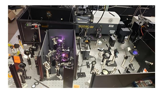
A laser apparatus built by SLAC lead scientist Matthias C. Hoffmann for experiments that shook ions traveling through a solid-state battery electrolyte with a jolt of voltage. To researchers' surprise, most of the ions responded by reversing course and hopping to their previous positions before returning to their usual erratic paths – the first indication that they remembered, in a sense, where they had been. Credit: Andrey D. Poletayev/Oxford University
