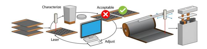
As part of NREL's BatMan project approach, researchers used computational simulations, advanced characterization, and laboratory-scale experimental prototyping to adjust and perfect the laser ablation technique for optimized results. Credit: Alfred Hicks, NREL
