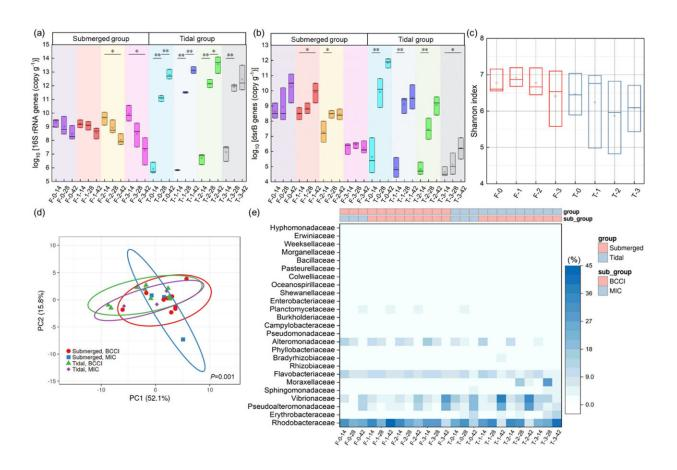
qPCR analysis of evolution for concentrations (copy g–1) of (a) 16S rRNA gene and (b) dsrB in concrete biofilms. Panel (c) is the α diversity of biofilm communities at the species level (Shannon index). Panel (d) shows differences in the microbial communities as visualized with PCoA. The permutational multivariate analysis of variance (PERMANOVA) was used to test differences
