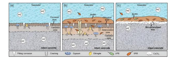
Corrosion mechanism for (a) chemical corrosion; (b) biofilm corrosion; (c) biomineralization for corrosion inhibition. Credit: 2024 Research and Innovation Office, The Hong Kong Polytechnic University. All Rights Reserved.
