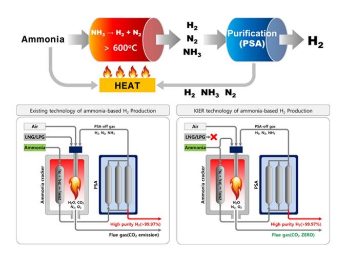
Basic principles of ammonia-based carbon-free hydrogen production technology (above). Credit: KOREA INSTITUTE OF ENERGY RESEARCH (KIER)
