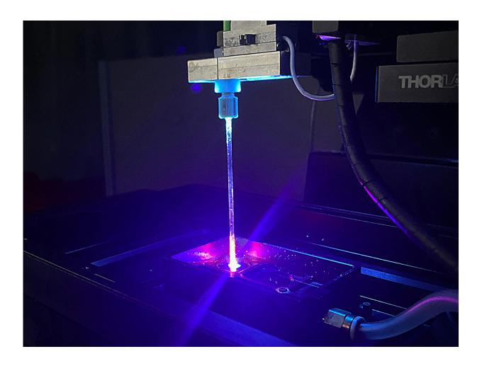
Test set-up with which the researchers tested how lime crystals adhere to different surfaces. Credit: Julian Schmid / ETH Zurich
