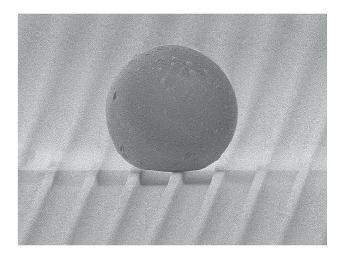
Test object polystyrene beads on the grooved surface. Credit: Julian Schmid / ETH Zurich
