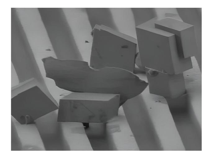
Only a few micrometer-sized lime crystals on the grooved surface under the electron microscope. Credit: Julian Schmid / ETH Zurich
