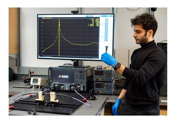
Omid Niksan holds a prototype of a 3D-printed MXene-coated component that can be used as an alternative for metallic components in antennas, waveguides and filters. Credit: UBCO
