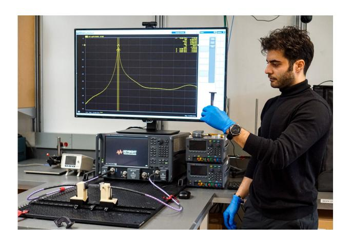
Omid Niksan holds a prototype of a 3D-printed MXene-coated component that can be used as an alternative for metallic components in antennas, waveguides and filters. Credit: UBCO
