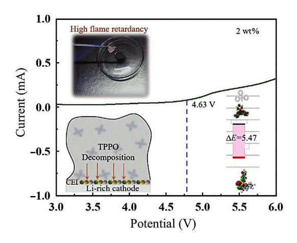
The increased oxidative decomposition potential is in evidence at 4.63 V allowing the potential formation of a passivation layer. The illustrations show the three most critical findings summarized; a high flame retardancy (upper left corner), the creation of a passivation layer on the cathode as TPPO decomposes
