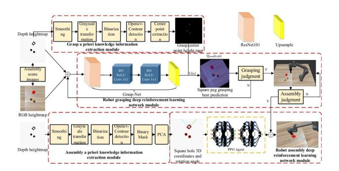
The diagram of the deep reinforcement learning method for robot grasping and assembly operation skills. Credit: *The International Journal of Advanced Manufacturing Technology* (2024). DOI: 10.1007/s00170-024-13004-0
