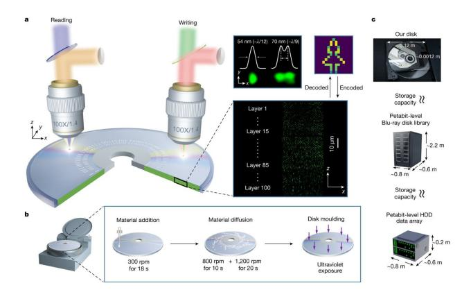
a, Dual-beam configuration for super-resolution writing and reading. b, Spin-coating process for material addition, material diffusion and blank-disk molding. c, The capacity of a single 3D nanoscale disk is approximately equivalent to that of a petabit-level Blu-ray library or an HDD data array. Credit: *Nature* (2024). DOI: 10.1038/s41586-023-06980-y
