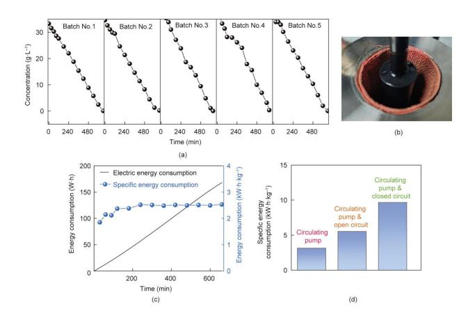
(a) Cu<sup>2+</sup> concentration change under different electrodeposition batches, (b) image of Cu recovered from TE&SF electrodeposition, (c) electric energy and specific energy consumption during electrodeposition, and (d) energy consumption of the entire process. Credit: Li Chen et al.
