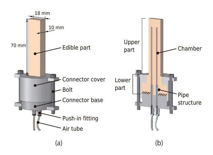
Three-dimensional computer-aided design model of the edible robot. (a) Edible robot and its (b) internal structure. Credit: *PLOS ONE* (2024). DOI: 10.1371/journal.pone.0296697
