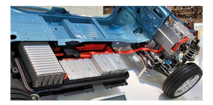
Cutaway view of a Nissan Leaf electric vehicle showing part of its battery array (silver boxes). Credit: <u>Tennen-gas/Wikipedia</u>, <u>CC BY-SA</u>
