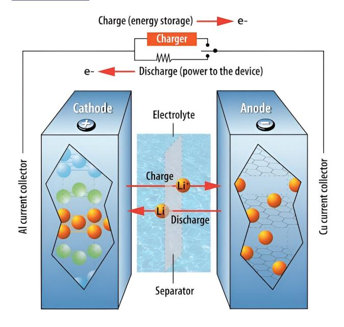
When a lithium-ion battery delivers energy to a device, lithium ions – atoms that carry an electrical charge – move from the anode to the cathode. The ions move in reverse when recharging. Credit: Argonne National Laboratory/Flickr, CC BY-NC-SA
