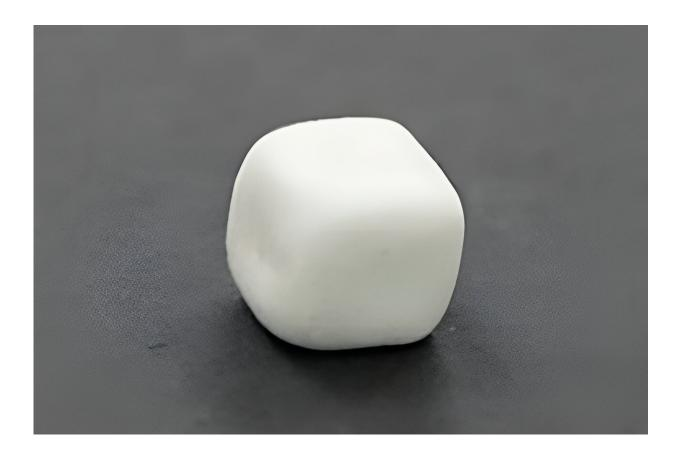
The gel-like electrolyte made of lithium chloride and gallium fluoride that shows promise of improving batteries. Credit: Samsung Advanced Institute of Technology
