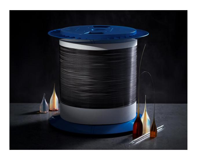
Hundreds of meters long high-performance flexible semiconductor fibers collected on a cylindrical bobbin, together with some preforms after the manufacturing process. Credit: Zhixun Wang
