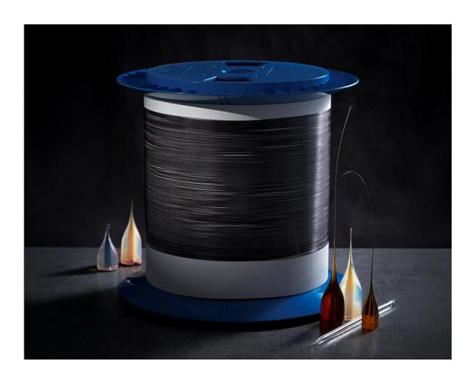
Hundreds of meters long high-performance flexible semiconductor fibers collected on a cylindrical bobbin, together with some preforms after the manufacturing process. Credit: Zhixun Wang
