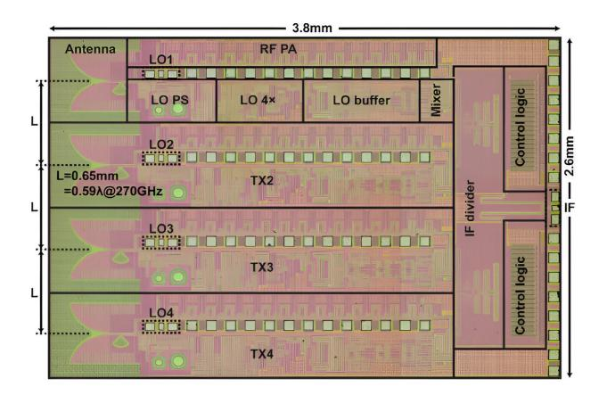
Chip die micrograph The proposed transmitter chip could pave the way for enhanced body and cell monitoring, radar, 6G wireless communications, and terahertz sensors. Credit: Tokyo Institute of Technology
