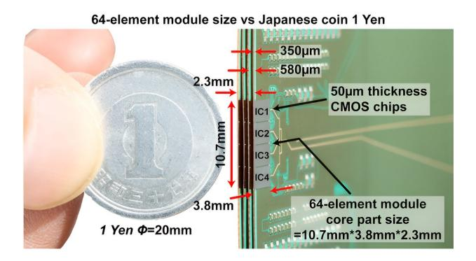
Compact phased-array transmitter with on-chip antennas Thanks to a highly optimized circuit topology and layout, the proposed transmitter chips can be arranged into a 64-element array occupying a minuscule volume. Credit: Tokyo Institute of Technology
