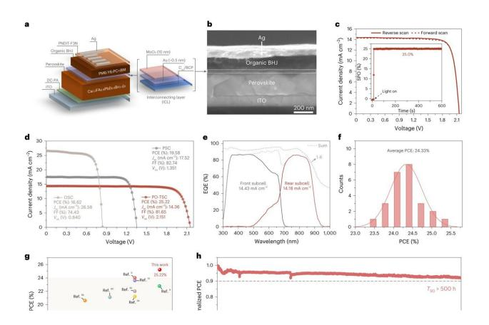
Photovoltaic performance of monolithic PO-TSCs. Credit: *Nature Energy* (2024). DOI: 10.1038/s41560-024-01451-8
