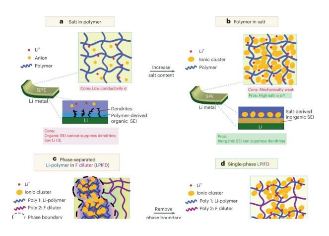
Schematic of the logic for designing single-phase solid polymer electrolytes based on polymer blends. Credit: *Nature Energy* (2024). DOI: 10.1038/s41560-023-01443-0
