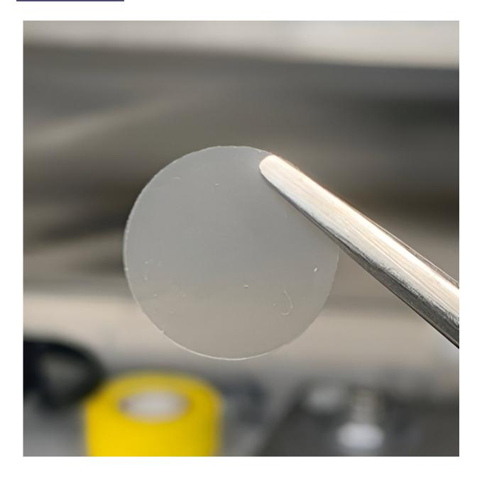
Image of solid polymer electrolytes. Credit: Zhang et al
