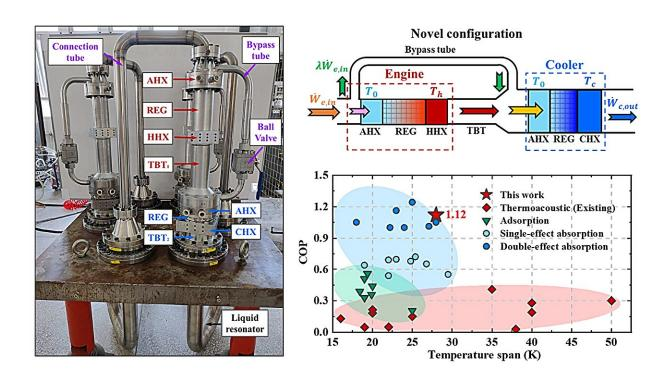
The developed novel heat-driven thermoacoustic refrigerator and its performance. Credit: TIPC
