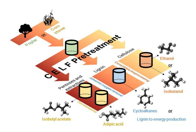
Simplified diagram for the proposed CELF-based biorefineries outlining the mass integration strategy. CELF: co-solvent enhanced lignocellulosic fractionation. Credit: *Energy & Environmental Science* (2023). DOI: 10.1039/D3EE02532B
