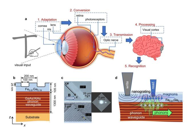
Nanodevice architecture and working principle. Credit: *Nature Communications* (2023). DOI: 10.1038/s41467-023-43891-y
