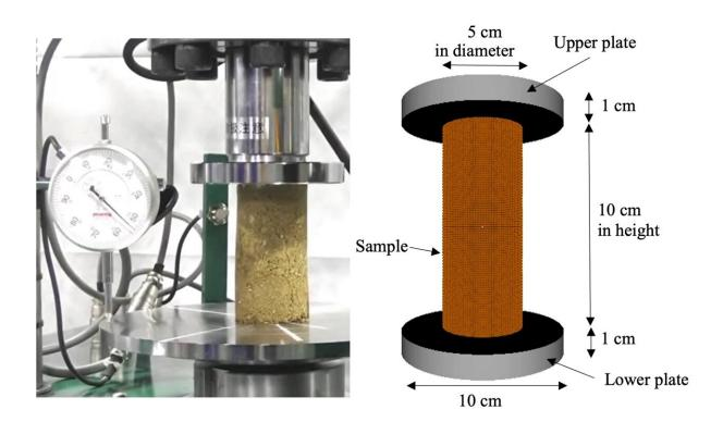
The goal of this study was to accurately match experimental data obtained from compression tests in particle-based simulations of soil behavior. Thanks to a comprehensive sensitivity analysis, the researchers shed light on the effects of several simulation and model parameters on the accuracy of the simulation results. Credit: Shinya Inazumi from Shibaura Institute of Technology
