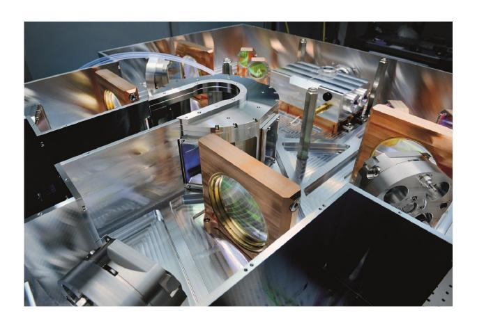
Gallium oxide crystals are produced in Japan with a 20 kW diode laser using the high-power optical system of the Fraunhofer ILT. Credit: Fraunhofer ILT, Aachen, Germany
