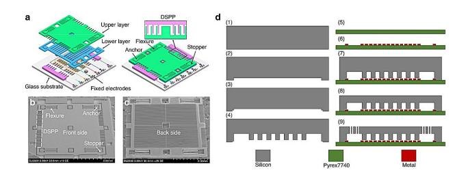
The design and fabrication of the proposed MEMS accelerometer. Credit: *Microsystems & Nanoengineering* (2024). DOI: 10.1038/s41378-023-00647-4
