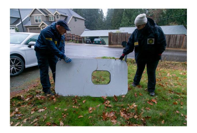
This photo released by the National Transportation Safety Board shows the door plug from Alaska Airlines Flight 1282 on Jan. 8, 2024, in Portland, Ore. Investigators say bolts that helped secure the panel on the Boeing jetliner were missing before the panel blew off the plane in midflight last month. The National Transportation Safety Board issued a preliminary report Tuesday, Feb. 6 into the Jan. 5 accident. The loss of the panel forced pilots of the Alaska Airlines Boeing
