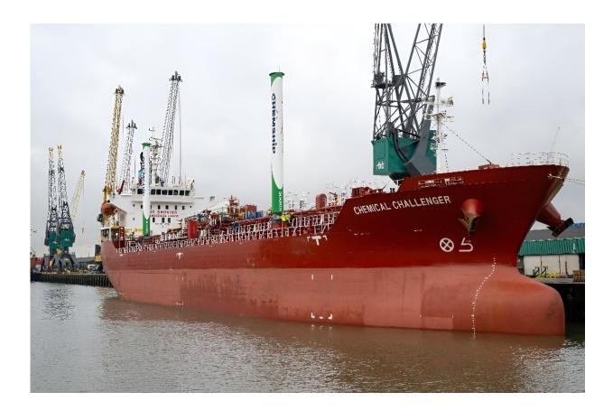
The four giant 16-metre-high sails similar to aircraft wings are hoped will cut fuel consumption by 10 to 20 percent.
