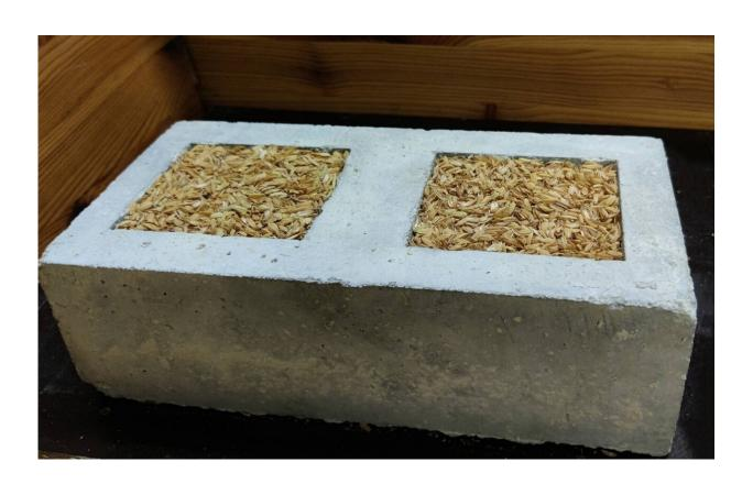
Concrete component made of recycled aggregates and rice husk ash with rice straw insulation. Credit: Fraunhofer-Gesellschaft
