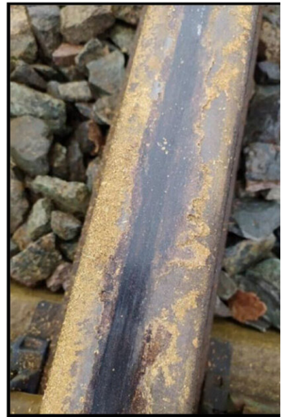
fully formed film (FFF) after braking passes
