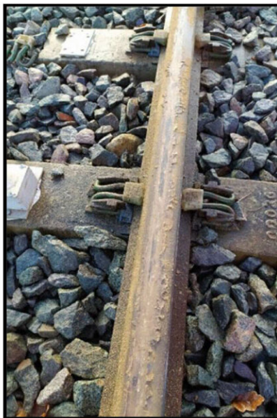
intermediate film (IMF) after rolling passes
