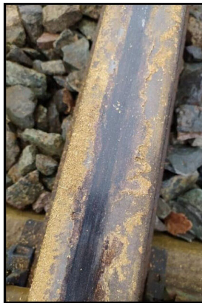
fully formed film (FFF) after braking passes
