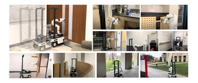
Open-World Mobile Manipulation System: We use a full-stack approach to operate articulated objects such as real-world doors, cabinets, drawers, and refrigerators in open-ended unstructured environments. Credit: *arXiv* (2024). DOI: 10.48550/arxiv.2401.14403
