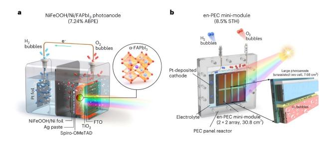
(a) Concept design of NiFeOOH/Ni/FAPbI<sub>3</sub> photoanode-based water splitting cell. (b) All-PSK-based encapsulated PEC reactor made of repeated minimodules (enlarged drawing). Credit: *Nature Energy* (2024). DOI: 10.1038/s41560-023-01438-x
