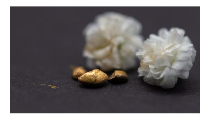
The gold nugget obtained from computer motherboards in three parts. The largest of these parts is around five millimeters wide. Credit: ETH Zurich / Alan Kovacevic
