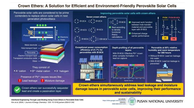
Researchers from Pusan National University show that crown ethers, specifically B18C6, can prevent lead leakage by forming strong host-guest bonds with lead ions in perovskite solar cells. They also provide higher resistance to degradation due to moisture. Credit: Ji-Youn Seo, Pusan National University
