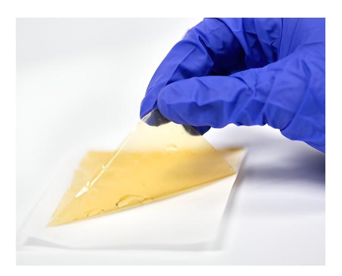
Scientists have successfully engineered a fatigue-resistant electrolyte membrane that exhibits resistance to cracking and significantly extends the lifespan of fuel cells. Credit: oakridgelabnews  $\underline{CC BY 2.0}$
