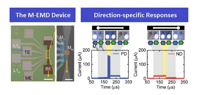
(Left) Optical image of the M-EMD device in the left panel (scale bar 200  $\mu$ m) and SEM image of the device in the right panel (scale bar: 20  $\mu$ m). (Middle) Responses of the M-EMD in positive direction. (Right) Responses of the M-EMD in negative direction. Credit: The Korea Advanced Institute of Science and Technology (KAIST)
